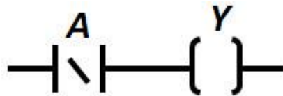
Figure 46. The ladder diagram NOT gate.
